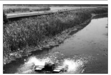
The Gyoutoku Bird Observatory's "Restoration of Shinhama: Cleaning the Water and Bringing Back Birdlife" won the fourth Research Contest in 1987. The photo shows a water wheel used to mix oxygen into the water, increasing the oxygen content of a polluted river.
